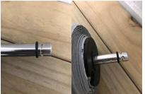
9. Slot into the idle end with the dimple on the pivot pin facing out to you.
